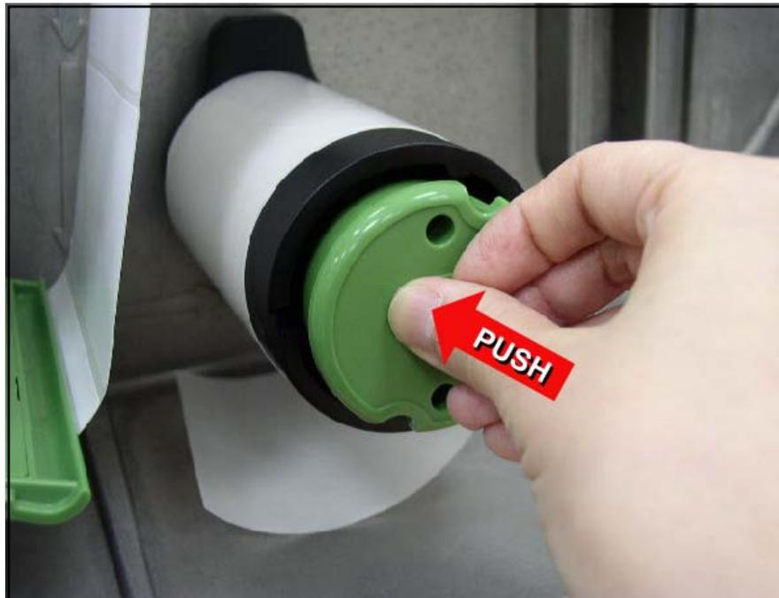
3. Then, slide off the liner from internal rewind spindle.
