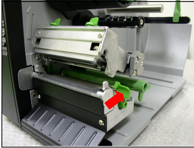
3. Insert the fan-fold media through the bottom or rear external label entrance chute.
