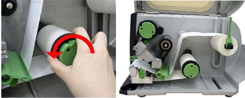
12. Lift up the peel-off roller release lever and close the print head mechanism.
