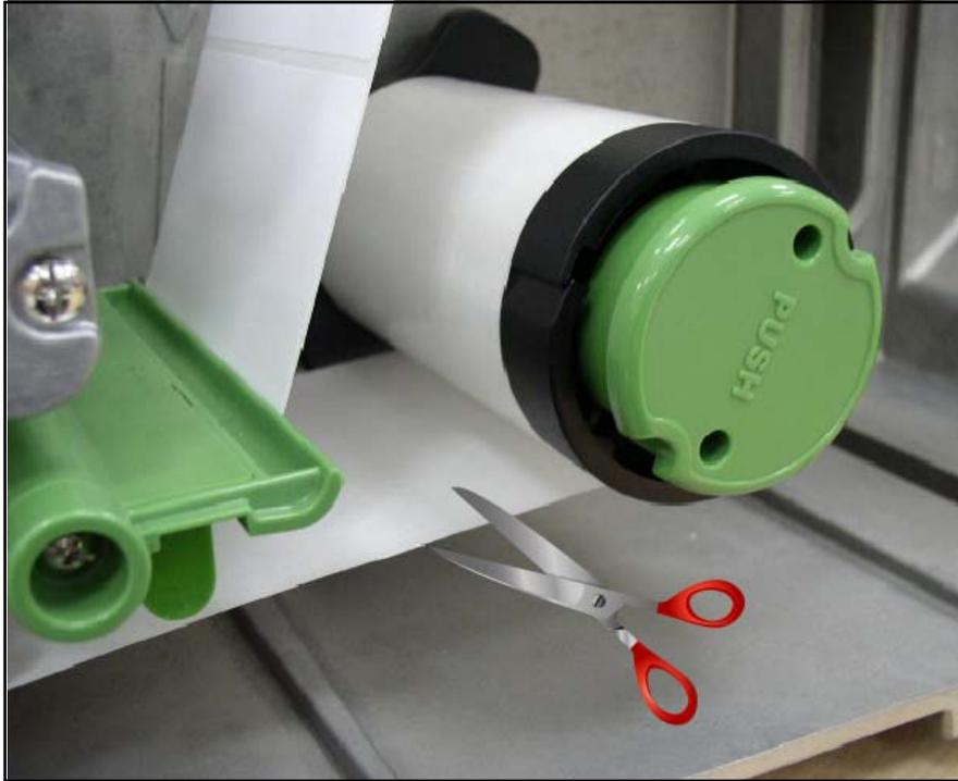
2. Push the liner release button to release the liner on the internal rewind spindle.
