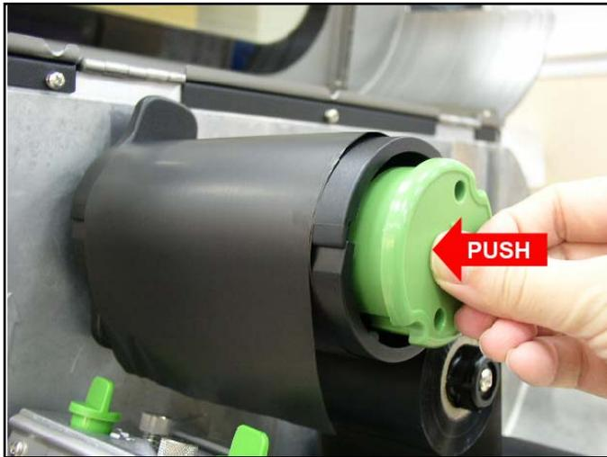
3. Then, slide off the ribbon from ribbon rewind spindle.
