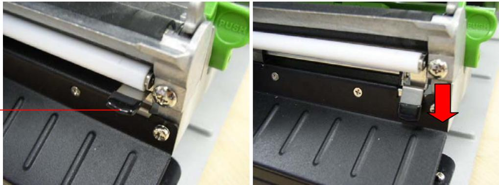
10. Feed the label between peel-off roller and platen roller.
