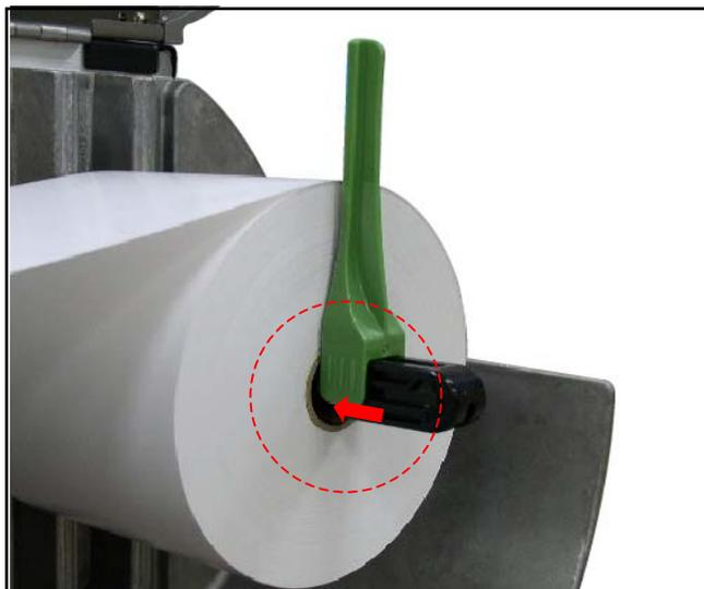
4. Pull label roll leading edge forward through the media guide bar, damper, media sensor and place the label leading edge onto the platen roller.
