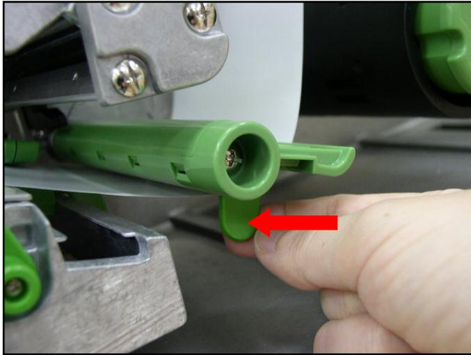
7. Close the print head mechanism making sure the latches are engaged properly.
