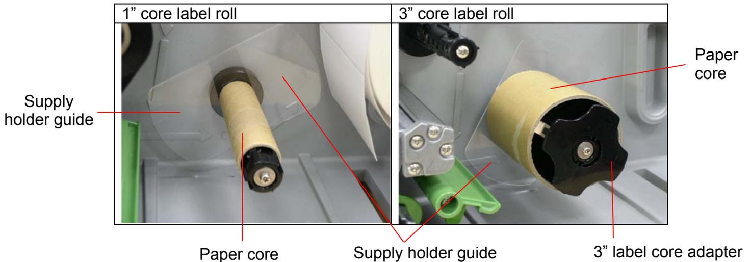
3. Insert media into the printer label spindle. Pull label roll leading edge forward through the media guide bar, damper media sensor and place the label leading edge onto the platen roller. (Please refer to section 2.6.1)
