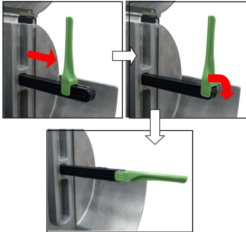
3. Place the roll of media on the label supply spindle. Flip up the label roll guard. Move the label roll guard horizontally to gently fit the width of label roll.
