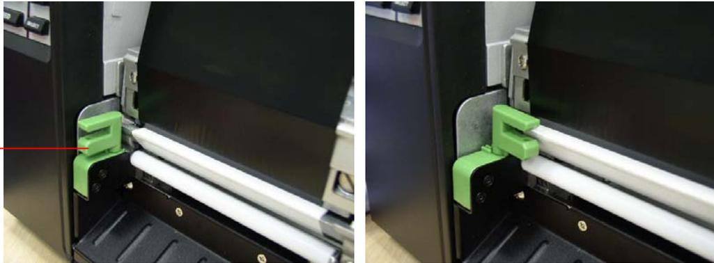
14. Peeling will automatically start. Press the FEED button to test.
