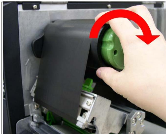
7. Close the print head mechanism making sure the latches are engaged properly.
