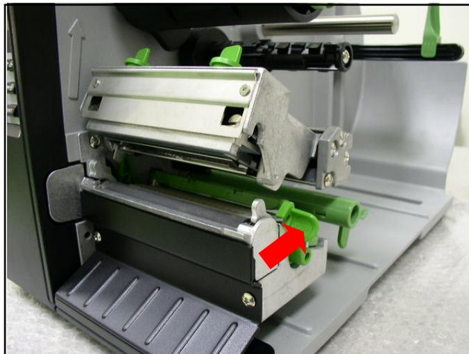
2. Move the label roll guard horizontally to the end of label spindle then flip down the label roll guard.
