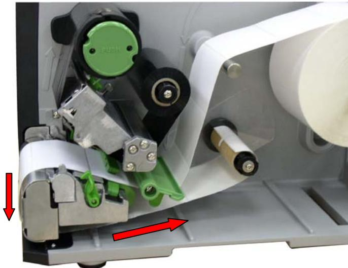
5. Insert another supply holder guide into the internal rewind for 1" core label roll.
