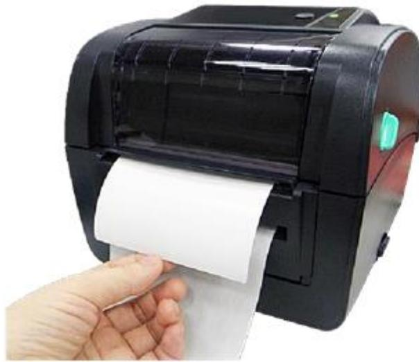
5. Disengage the top cover support to close the top cover. Printer is ready for peel-off mode.
