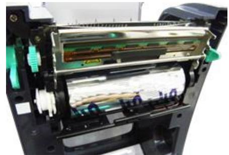
4. Insert the paper core right side onto the rewind hub. Align the notches on the left side and mount onto the spokes.
