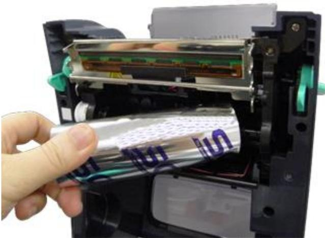
3. Insert the ribbon right side onto the supply hub. Align the notches on the left side and mount onto the spokes.
