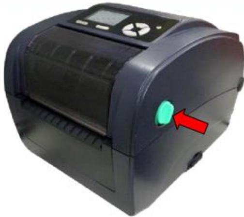
1. Open the printer's top cover by pulling the top cover open levers located on each side of the printer and lifting the top cover to the maximum open angle.
