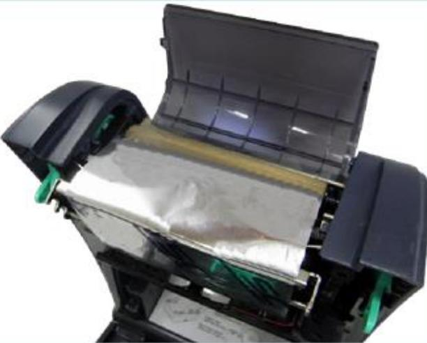
5. Stick the ribbon onto the ribbon rewind paper core. Additional tape may be required.
