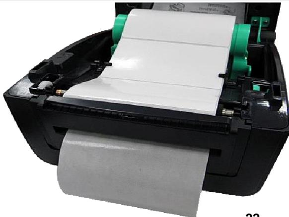
4. Close the peel-off module. Use the DiagTool or LCD menu function to enable the peel-off mode.
