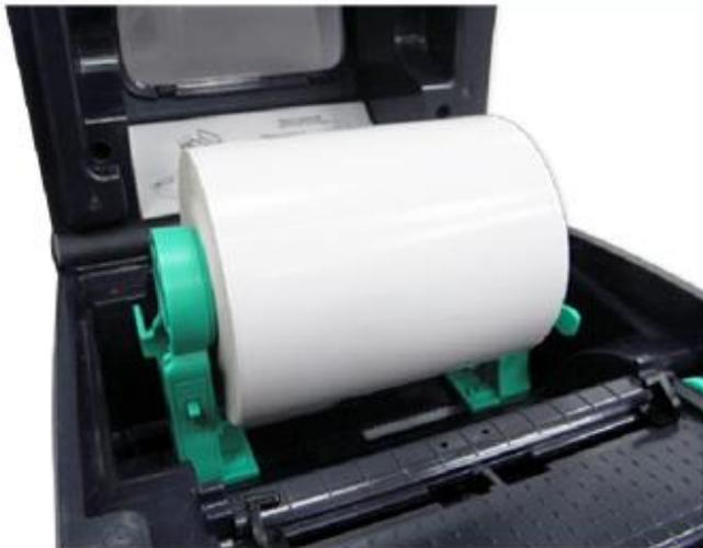
3. Place the roll between the holders and close them onto the core.
