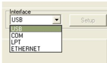
5. Click on the Printer Function “Ethernet Setup” button. DHCP is the default. Select “Static IP” to assign the IP address, subnet mask and gateway for the on board Ethernet.
