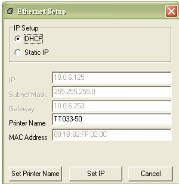
The default IP address is obtained by DHCP. To change the setting to static IP address, click “Static IP” radio button then enter the IP address, subnet mask and gateway. Click “Set IP” to take effect the settings.
