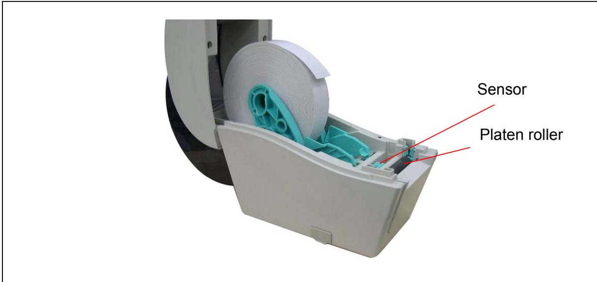
4. Place the media, printing side face up, through the media guides, over media sensor and place the label leading edge onto the platen roller.
