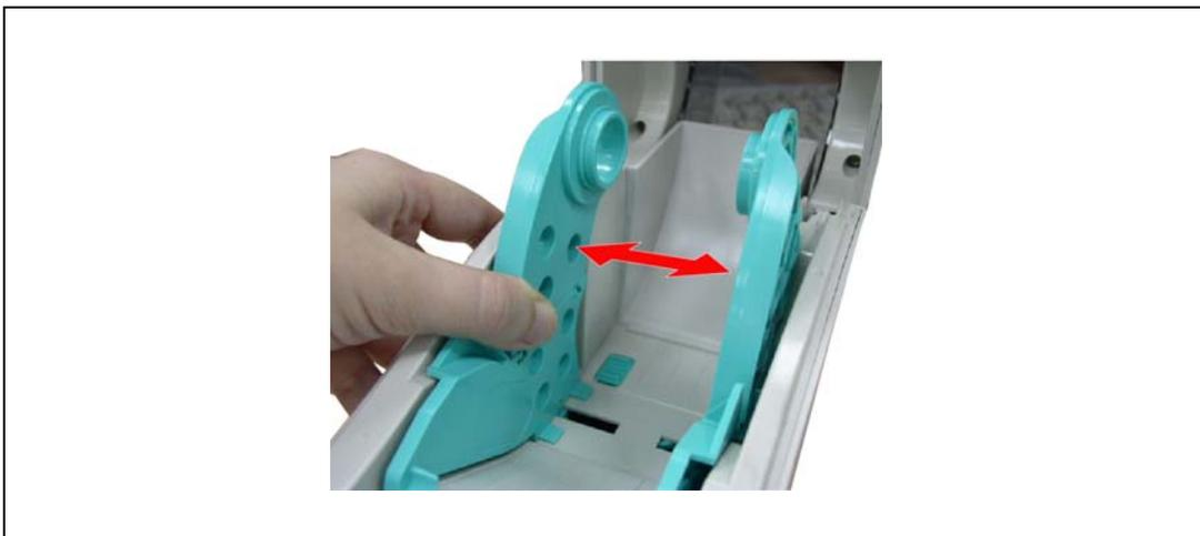
3. Place the roll between the holders and close them onto the core.
