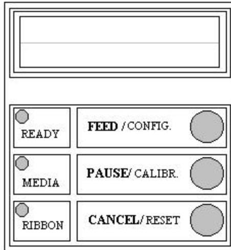
**Figure 23 - Fastmark 4000 Series Front Panel**
