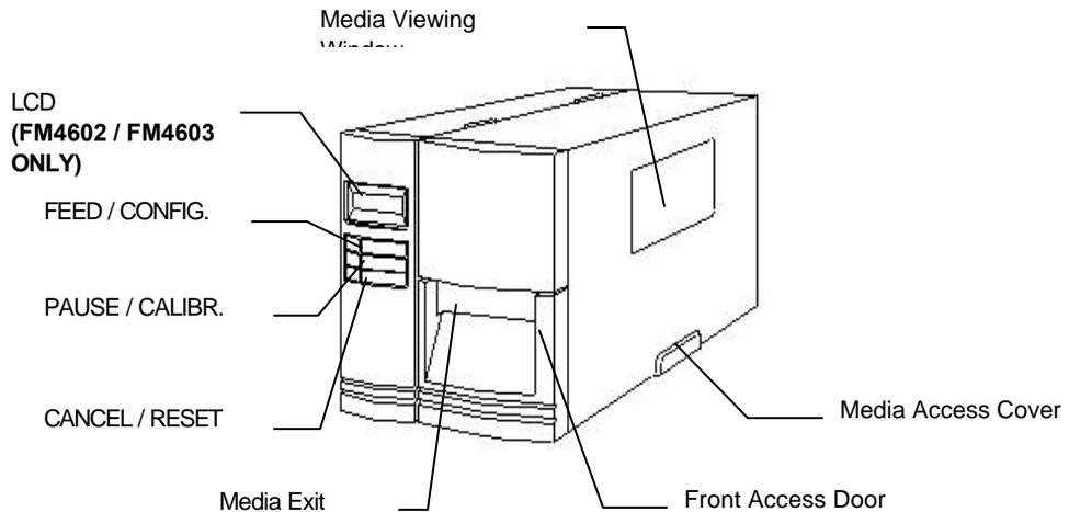
**Figure 4 - Front and Side View**
