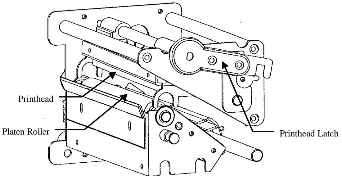
**Figure 27 - Printhead (TPH) Maintenance**
