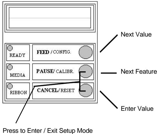
**Figure 24 - Entering into Set-up Mode**
