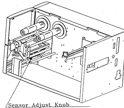
**Figure 16 - Media Sensor Adjust Knob**
