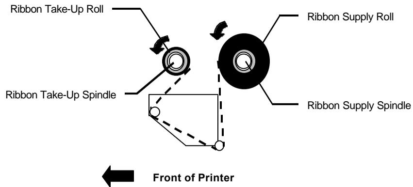
**Figure 12 - Ribbon Routing**
