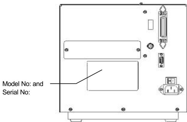
**Figure 2 - Model and Serial Number Location**
