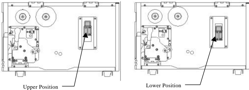
**Figure 18 - Media Spindle Location**
